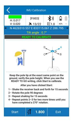
The calibration consists of the same movement repeated along the four orthogonal directions while keeping the pole tip on the same point on the ground:
